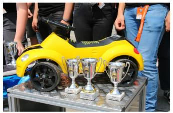
car. In the summer of 2019, a group of 8 apprentices from different professions, including myself, got the chance to construct and build their very own car in the size of a bobby car. It was powered by a cordless drill and controlled with an Arduino and remote control. The car was able to go up to 45km/h and tow over
